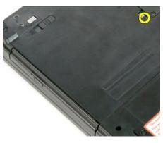
4. Insert a plastic scribe into the notch and slide the optical drive slightly out of the computer.
