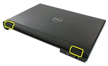
4. Starting on the right side, separate the hinge cover from the base of the computer.
