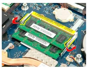
5. Slide the memory module out of the socket.
