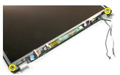
5. Remove the LCD display panel from the display assembly.
