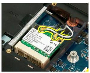
5. Remove the screw that secures the WLAN card to the computer.
