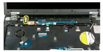
10. Remove the four remaining screws that secure the display assembly to the computer chassis.
