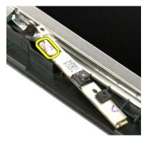
7. Remove the camera from the display assembly.
