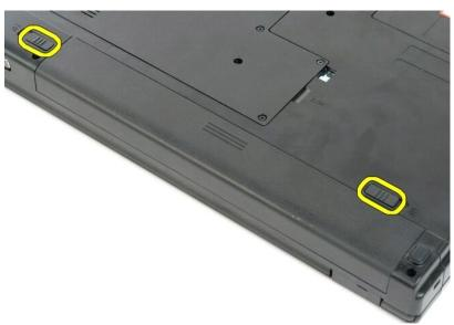
3. Slide the battery toward the back of the computer to remove.
