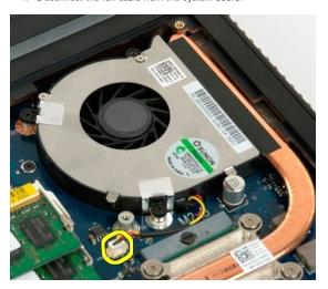
5. Remove the three fan screws.
