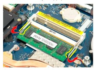
7. Slide the memory module out of the socket.
