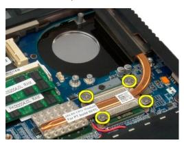
6. Lift the edge of the heat sink that is closest to the center of system board.
