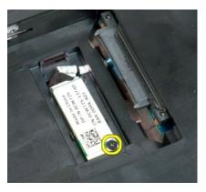
5. Lift the edge of the Bluetooth module closest to the front of the computer.
