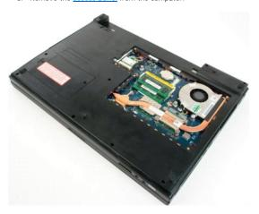
4. If applicable, remove the top memory module by using your fingertips to carefully spread apart the securing clips on each end of the top memory module connector until the memory module pops up.
