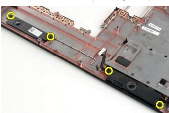
13. Remove the speaker assembly from the computer.
