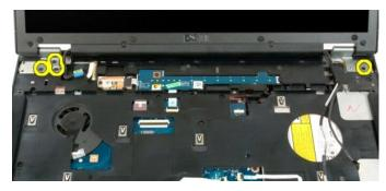
11. Lift the display assembly straight up and remove the display assembly from the computer.
