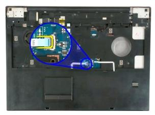
9. Open the fingerprint reader data cable clip.
