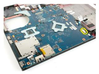
13. Disconnect the Bluetooth® module cable from the system board.
