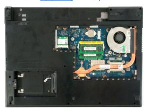
6. Remove the eleven palm rest screws that secure the palm rest to the bottom of the computer.
