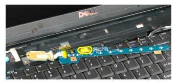
10. Remove the two button pads from the computer.
