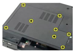
4. Lift the edge of the access panel that is closest to the center of the computer.
