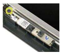
5. Lift the camera from the retention bracket.
