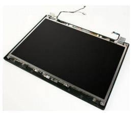
4. Remove the screw that secures the camera to the display assembly.
