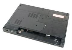
3. Remove the eight screws from the access panel.
