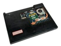
4. Disconnect the fan cable from the system board.
