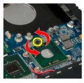
9. Lift the processor straight up from its socket, taking care not to bend any of the processor pins.
