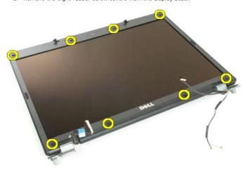
4. Remove the eight screws that secure the bezel to the display assembly.
