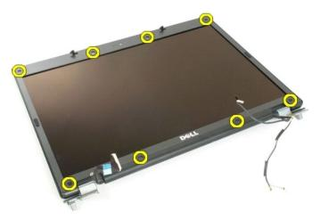
5. Remove the bezel from the display assembly.
