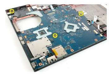
16. Remove the system board from the computer chassis.
