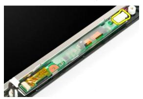
5. Remove the inverter from the display assembly.
