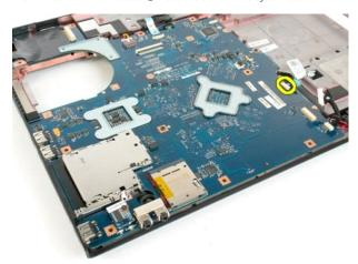
14. Disconnect the power cable from the system board.
