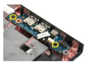
13. Lift the inside edge of the USB board and remove the board from the computer.
