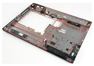
12. Remove the four screws that secure the speaker assembly to the computer chassis.
