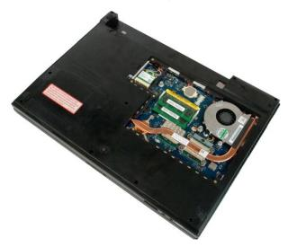
4. Disconnect the antenna cables from the WLAN card.
