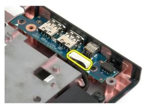
12. Remove the two screws that secure the USB board to the computer chassis.
