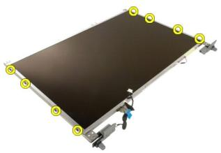
6. Slide the hinges away from the display panel assembly.
