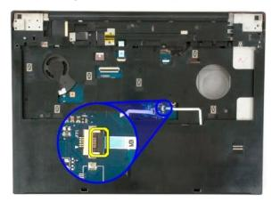
10. Remove the fingerprint reader data cable from the clip.
