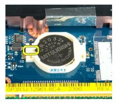
5. Remove the coin-cell battery.
