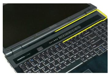
$5. \quad \text{Continue to separate the hinge cover from the system working from right to left, then remove the hinge cover.} \\$
