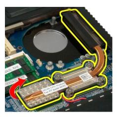
7. Slide the heat sink toward the center of the computer, then lift up the heat sink and remove it from the computer.
