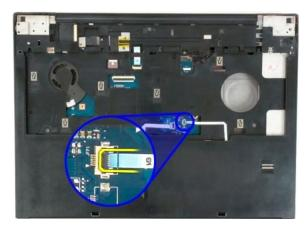
11. Remove the nine palm rest screws that secure the palm rest to the top of the computer.
