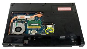
6. Remove the three screws that secure the display assembly to the computer chassis.
