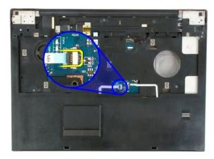
8. Remove the touch pad data cable from the clip.
