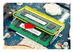
6. If applicable, remove the bottom memory module by using your fingertips to carefully spread apart the securing clips on each end of the memory module connector until the memory module pops up.
