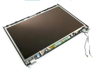
4. Remove the two screws that secure the LCD display panel to the display assembly.
