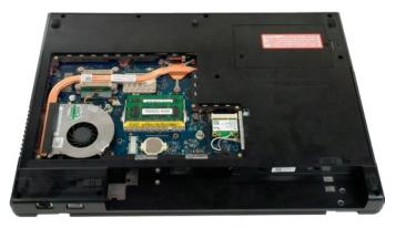
5. Disconnect the antenna cables from the WLAN card.
