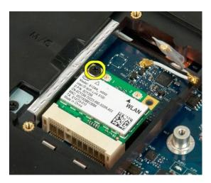
6. Remove the WLAN card from the computer.
