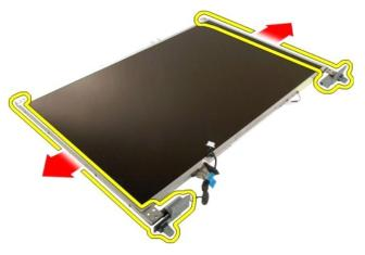
7. Remove the display panel hinges from the display panel assembly.
